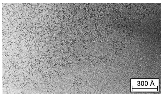
Fig. 5. Transmission electron micrograph of the precipitate (see Section 4.4), recovered from the catalytic cyclohexene autoxidation reaction in the presence of the catalyst precursor [n\text{-Bu}_4\text{N}]_5\text{Na}_3[(1,5\text{-COD})\text{Ir}\cdot\text{P}_2\text{W}_{15}\text{Nb}_3\text{O}_{62}] , 1 , redissolved in acetonitrile and applied to a carbon-coated Cu TEM grid.
